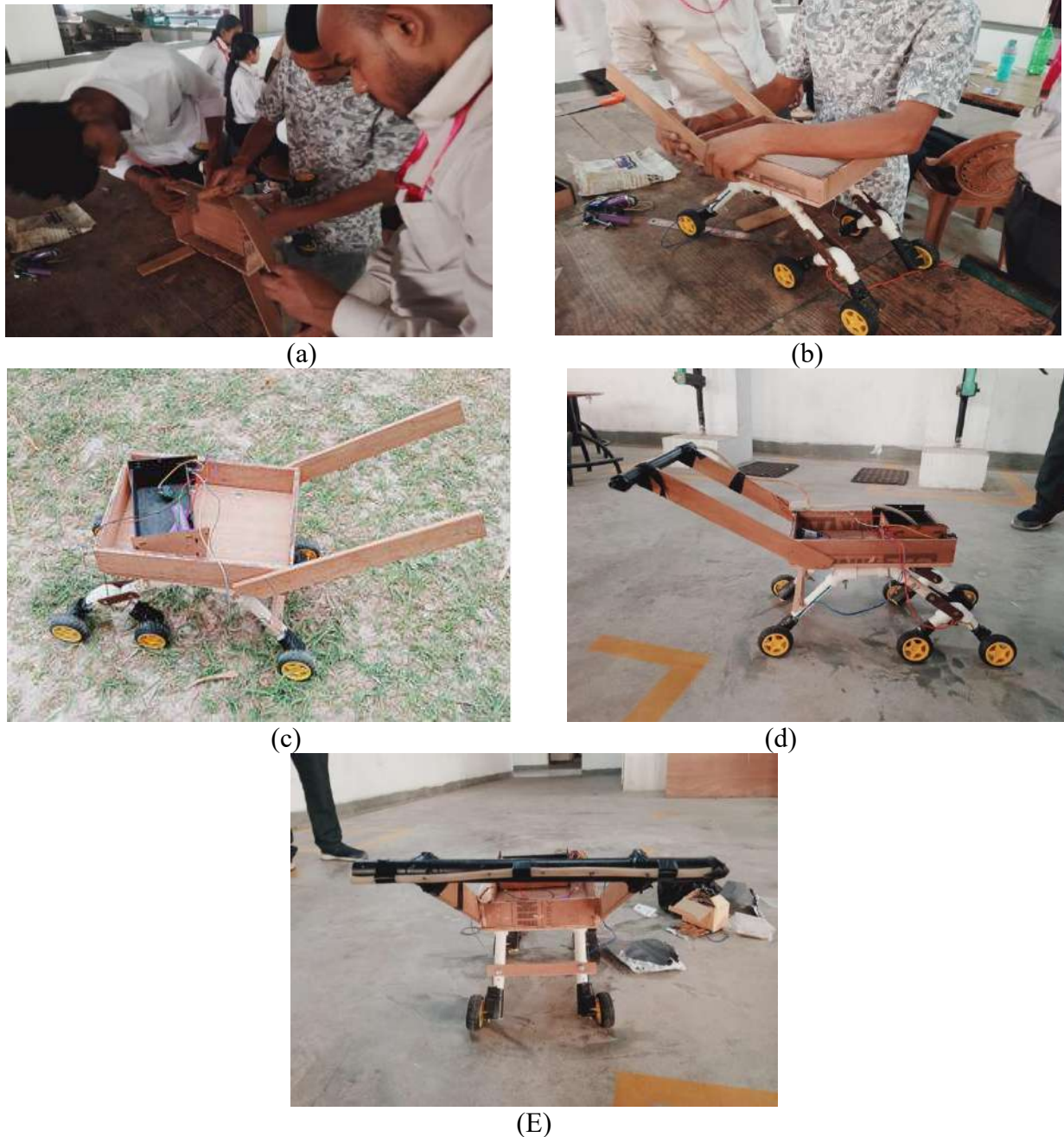
Figure 2 Sequential Fabrication Images of the Chassis Assembly, Rocker-Bogie Linkage Construction, Wheel Mounting and Spray Pipe Integration
